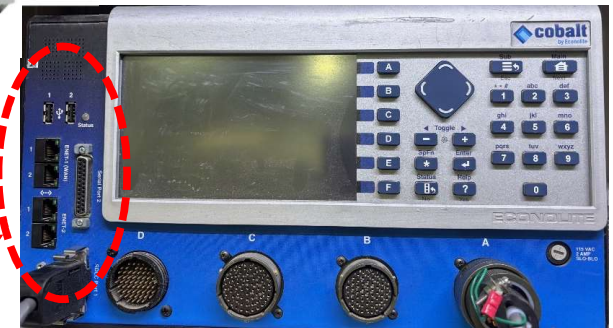
TS-2 Type 2 Controllers With Ethernet Port that serves to connect to fiber
