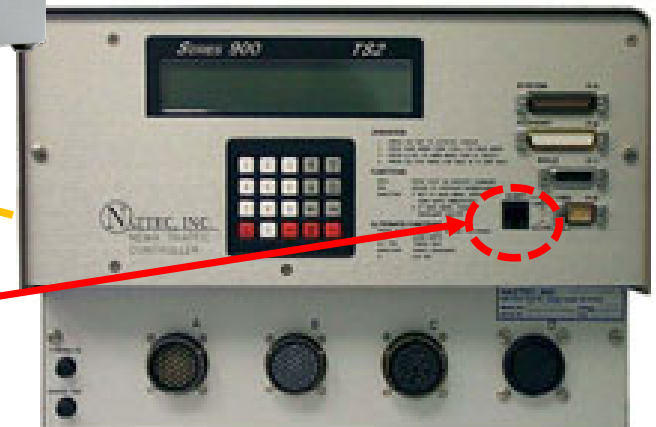
TS-2 Type 2 Controllers With Ethernet Port that serves to connect to fiber
